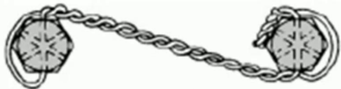
Safety wire Bolt-Heads
