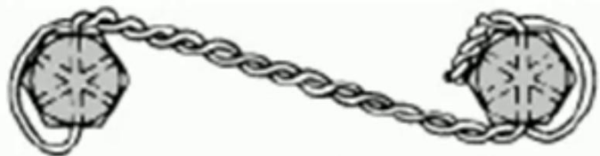
Safety wire Bolt-Heads
